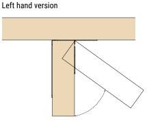
Rotate hanger to angle required. Correct hand must be used. Please ensure the correct hanger has been selected prior to installing.
