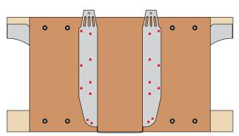
Position hanger flush with underside of joist.
