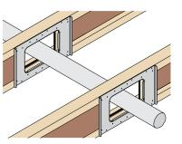
Plate required each side of aperture.
