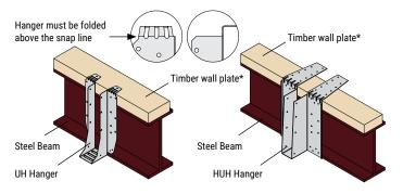
Characteristic Hange Hanger Hanger Capacity (kN) Depth Width Face Тор Incoming Туре (mm) (mm) Uplift Down 195 4 2 2 1.98 10.80 UH 39-100 220/235/ 4 2 4 3.97 10.80 300 HUH 39-300 6 6 4 3.97 13.20 All depths
