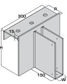
M-RTN-THICKNESS-W-H-R Example: M-RTN-8MM-100-225-100
