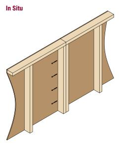
PSTS to be fixed at panel joints to engineer's specification.
