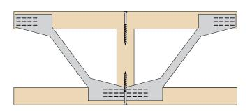
Vertical blocking piece to be built into Open Web Joist, centred on incoming hanger position.
