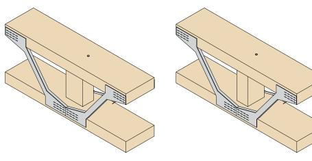
Applying a high load to the top flange of an open web joist can lead to failure of the joist itself (i.e metal webs buckling)
