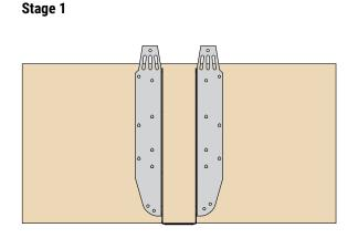
Position hanger against face of joist with locating tab tight to underside of joist.
