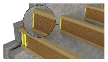
Mortar cavity side to achieve 60 minute Fire Rating and air tightness performance.
