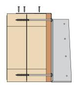
Nail top tabs into top chord of joist – Min 2No  $3.4 \times 35$ mm square twist nails into rear ply and 1No  $3.4 \times 35$ mm square twist nail into front ply per leg.
