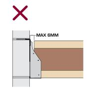
Do not install the hanger with a gap exceeding 6mm between the joist/truss and the hanger.
