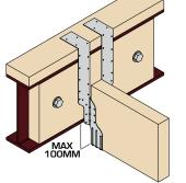
The KHL hanger is a long leg hanger designed for simple solid timber to timber connections.
