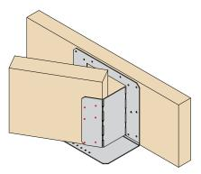
Please ensure that 1No inner nail hole (indicated in red) and 1No outer nail hole (indicated in red) are filled on the underside with 3.4 x 35mm square twist nails.
