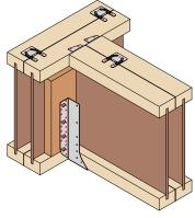
Offer incoming member into the MHE hanger and fix to joist bottom flange/ backer block and UZ-Clip to header member.
