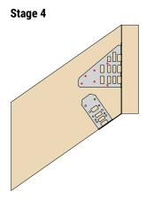
Wipe round the top side flange at the appropriate crease line and fill all the nail holes into the incoming joist. Minimum 4No 3.4 x 35mm square twist nails.
