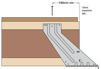
Minimum edge distance for decking nails = 150mm
