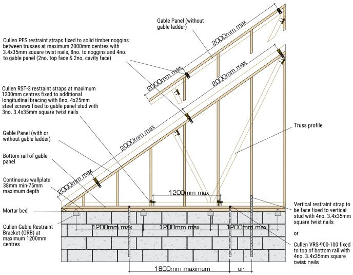
Vertical restraint strap plugged and screwed to blockwork at maximum 1.8m centres, either: Cullen VRS-900-100 installed to top of gable panel bottom rail or
