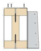
Nail top tabs into top chord of joist – Min 2No  $3.4 \times 35$ mm square twist nails into rear ply and 1No  $3.4 \times 35$ mm square twist nail into front ply per leg.
