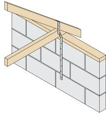
RST strap to be nailed to truss with 3.4 x 35mm square twist nails. Nail quantity dependant on uplift value. Fixings into masonry to be specified by building designer.
