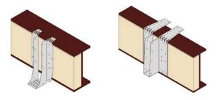
Hanger fixed directly to top flange of steel beam using 4no. Spit Spitfire P370 Cartridge tool using SC9 nails or equivalent, into the hanger flanges. Hanger fixed to timber packer secured to web of steel beam using 3.4 x 35mm square twist nails. Timber packer fixed to web of beam (as per Building Designers instructions) to prevent hanger rotation. Timber packers must be a minimum of 35 x 72mm C16 grade timber.
