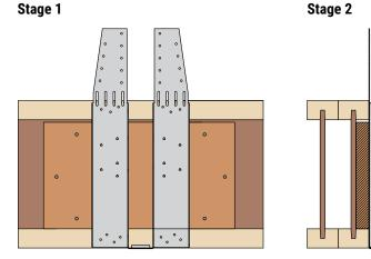
Position hanger flush with underside of joist.
