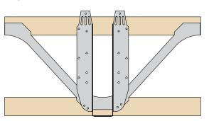
Position hanger against face of open web joist with locating tab tight to underside of joist.
