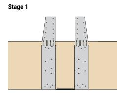
Position hanger flush with underside of joist.
