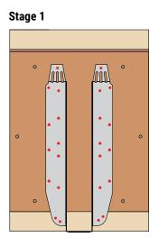
Position hanger against face of I–Joist with locating tab tight to underside of joist.
