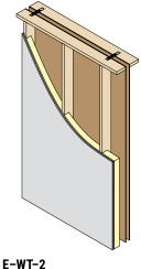
(timber frame cavity wall with sheathing)
