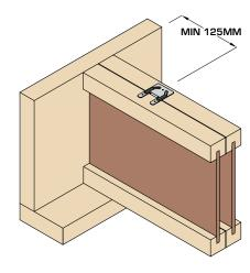
Installation on joist end to be minimum 125mm away from the end of the joist to allow adequate space for fixing.
