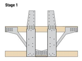
Position hanger flush with underside of joist.
