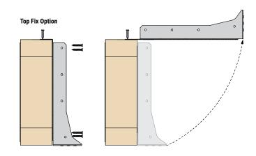
Face fix to top and bottom chords using 8No screws or nails. Bend top tabs over joist top flange and nail using 1No fixing per leg. Once ready for stairs to be installed the deck can be cut and joists/ hangers removed.
