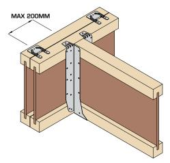
Installation either side of incoming point load to be maximum 200mm from joist edge.
