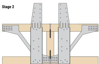
Position hanger against face of Open Web Joist with locating tab tight to underside of joist.
