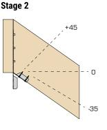
Offer incoming member and fix using 2No 3.4 x 35mm square twist nails to the underside of the incoming member.
