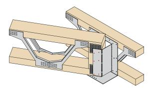
Please ensure that 1No inner nail hole (indicated in red) and 1No outer nail hole (indicated in red) are filled on the underside with 3.4 x 35mm square twist nails.
