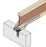
Lateral restraint of the walls can be provided by the floor, the restraint must be provided parallel and perpendicular to the floor joists.
