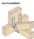
The TS hanger is designed to support trussed rafters from primary girders.
