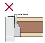
Do not install the hanger with a gap exceeding 6mm between the joist/truss and the hanger.
