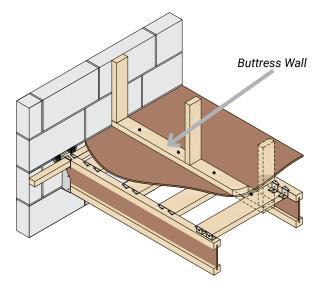
Buttress wall can be positioned off-centre on the noggins.
