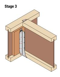
Fix UZ-Clip to top flange of supported member using:
