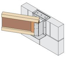
Ensure that 1No inner nail hole (indicated in red) and 1No outer nail hole (indicated in red) are filled on the underside with a 3.4 x 35mm square twist nail.
