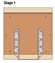
Position hanger against face of I–Joist with locating tab tight to underside of joist.
