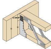
Applies to MHE/MHI/MHIC – Hanger height (H) must be minimum 60% of joist depth (D).
