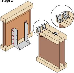
Fix UZ-Clips to top flange of supported member using:
