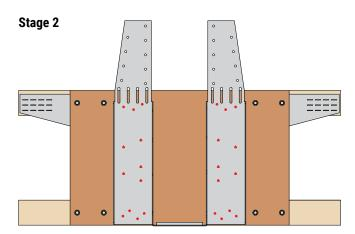
Position hanger flush with underside of joist.
