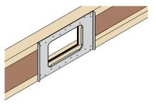
Position SHI plate at least 90mm from joist end to ensure it does not clash with masonry hanger or end seal (suitable for use
