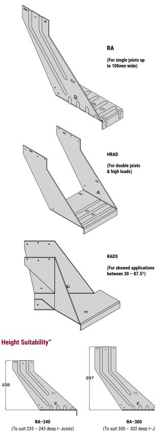
(To suit 300 - 302 deep I-Joists) (To suit 304 deep Open Web Joists)
