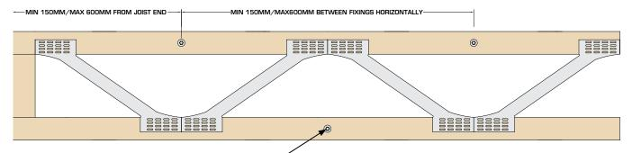
PSTS screws should be installed into both top and bottom chords ensuring a fastener is located within each V section.
