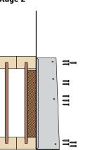
Fill all round and triangular nail holes to header and backer face with 3.4 x 35mm square twist nails.
