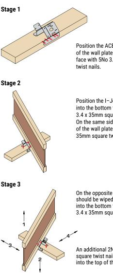
Position the ACE to the outside of the wall plate and nail to the face with 5No 3.4 x 35mm square
