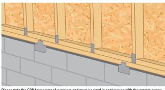
Please note the GRB forms part of a system and must be used in conjunction with the system straps and fixings as shown on Pages 132-133
