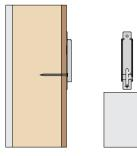
Nail channel into wall panel by nailing 1No fixing at the bottom of the slot. Allow adequate space above the masonry to hammer fix.
