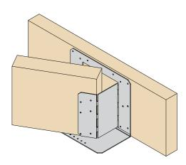
Solid timber joists must be full depth of hanger
