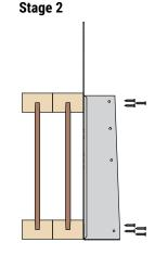
Position hanger flush with underside of joist.
