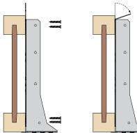
Face fix to top and bottom flanges using 8No 3.5 x 30mm multi purpose wood screws or 3.4 x 35mm square twist nails.
