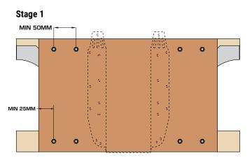
18mm plywood should be fixed to the face of the open web joist with 4No PSTS 6.5mm into the top chord and 4No PSTS 6.5mm into the bottom chord.
