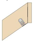
Wipe up the bottom side flange at the appropriate crease line and fill the 2No nail holes closest to the bend line with 3.4 x 35mm square twist nails.
