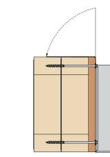
Wipe over top tabs to give a flush fit to the joist.
