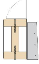
Wipe over top tabs to give a flush fit to the joist.
