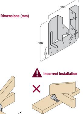
Do not install truss clips horizontally onto the wall plate.
