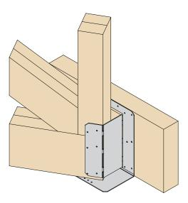
Bottom chord must be deeper than hanger or vertical required for trusses
