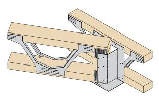
Adequate end blocking required to allow fixings into incoming Open Web Joist
