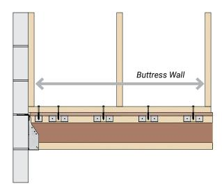
Noggins are evenly spaced between the joists (excluding perimeter noggin) and installed using UZ clips.
