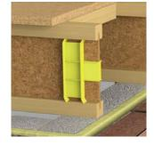
Place the Hi–Vis Gripper onto one end of the I–Joist to be built into the masonry. Push fit until it is fully engaged. Ensure it tightly abuts the I–Joist web and that both ends of the Hi–Vis Gripper tightly abut the I–Joist flanges.
