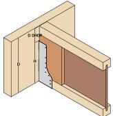
Applies to MHE/MHI/MHIC – Hanger height (H) must be minimum 60% of joist depth (D). Where hanger drop (D DROP) exceeds values below web stiffeners are required.
