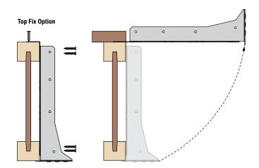
Face fix to top and bottom flanges using 8No 3.5 x 30mm multi purpose wood screws or 3.4 x 35mm square twist nails.
