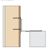
Position channel by lightly tapping with a hammer until channel is in correct position.
