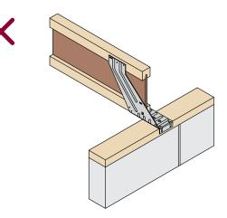
Do not install the RA range onto a timber wall plate.
